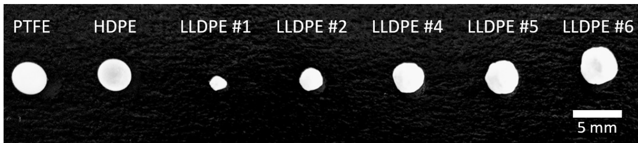
Figure 3-1: Array of particles used for the charge generation experiments.
