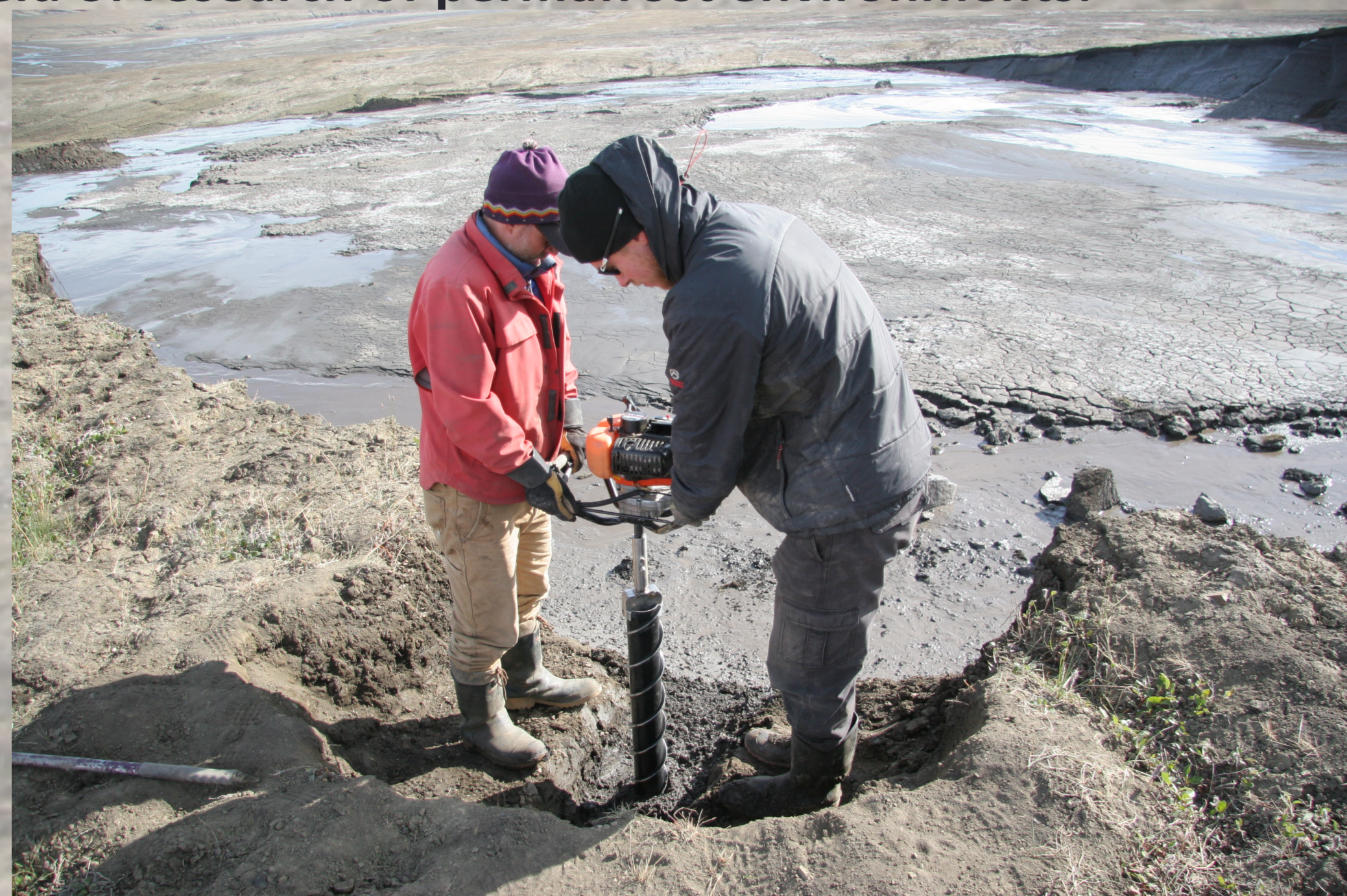
Figure 3: Coring process during field work in Eureka. Source: Professor Wayne H. Pollard
