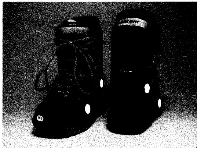
Figure 3-8: Location of the holes drilled in the snowboard boot, shown here on a boots similar to those used in the present project (adapted from www.rakuten.co.jp ). One-centimetre diameter holes for anatomical landmark measurements are shown in yellow. The four-centimetre diameter hole to let the foot sensor stick out is shown in red.
