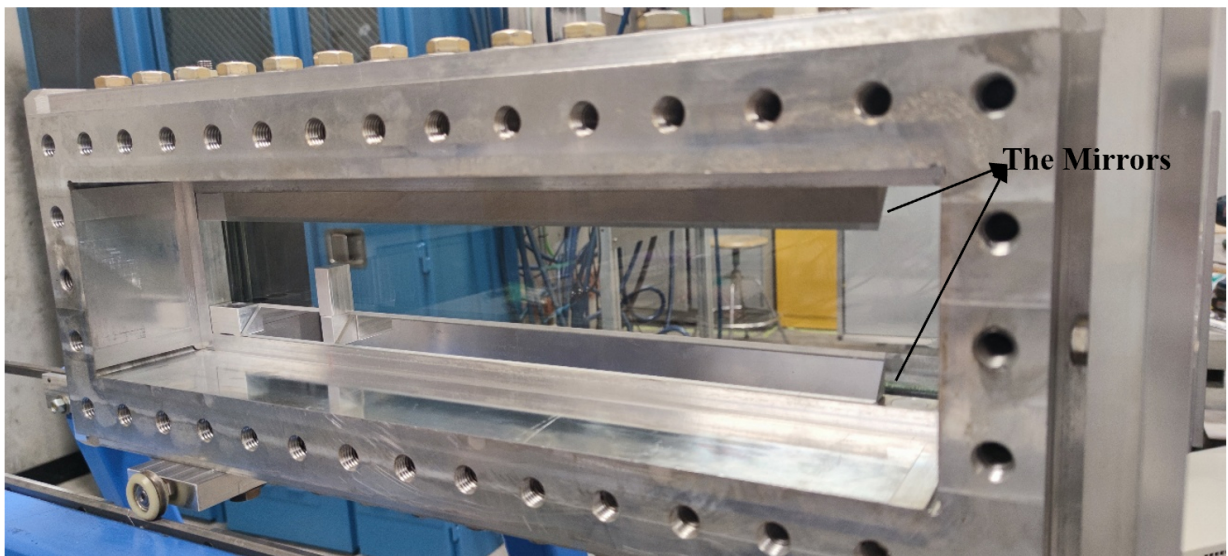
Figure 2.6: Mirrors configuration inside the shock tube for three-dimensional visualization
