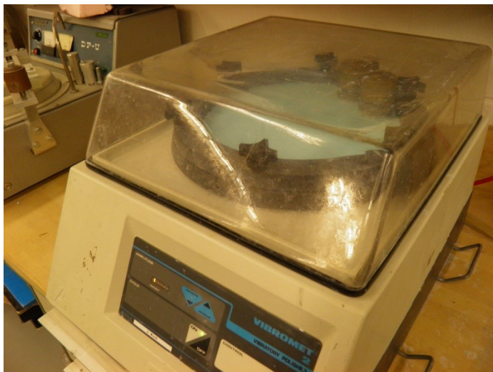
Figure 34: Vibratory Polisher (with blue polishing suspension and two samples)
