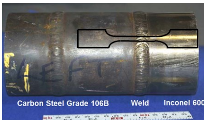
Figure 38: Large Tensile Sample Location and Dimensions
