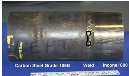
Figure 41: Miniature Tensile Sample Location and Dimensions
