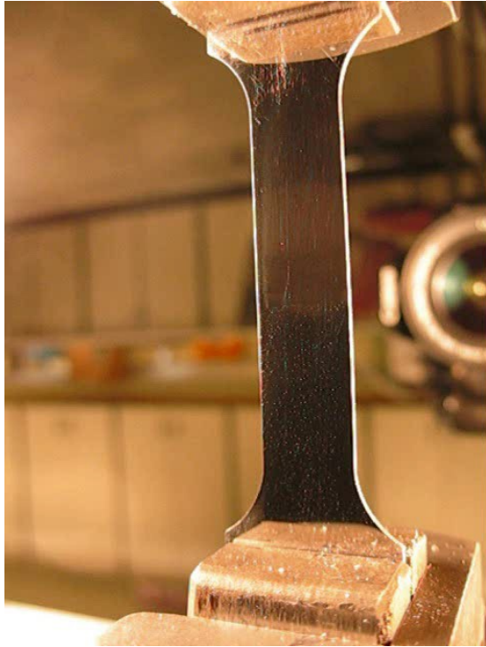
Figure 39: Large Scale Tensile Test Set-Up viewed from Polished Side
