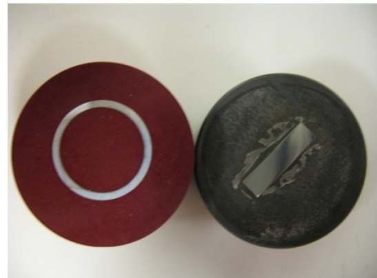
Figure 45: Mounting Options. Left - Cylindrical sample mounted in resin. Right - Miniature Tensile Sample glue to cylindrical puck as completed in this project.
