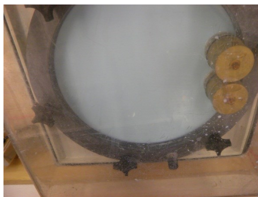
Figure 35: Vibratory Polisher From Above (samples are under brass cylinders which are used for weight)
