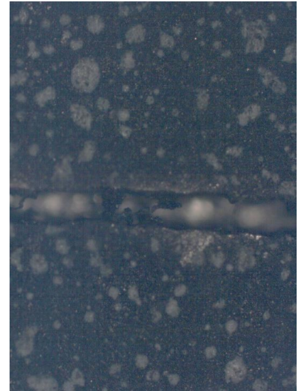
Figure 75: Crack in sample 3B (Image Under 5x microscope)
