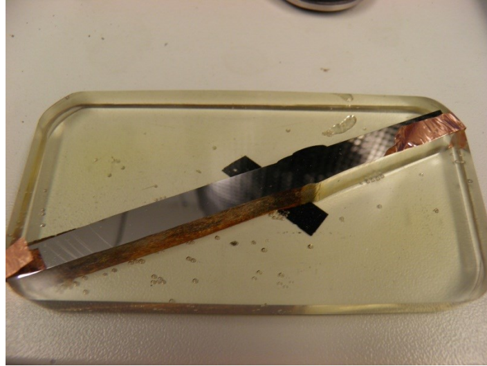
Figure 37: EDS sample, note copper tape glued to the sample to increase conduction
