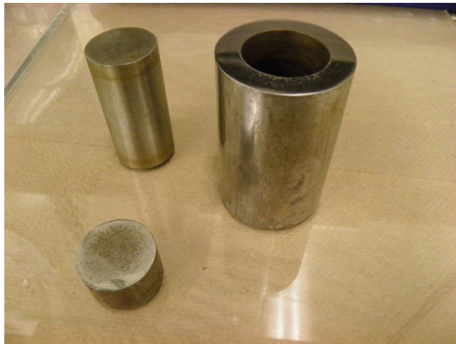
Figure 44: Polishing Apparatus for Miniature Samples. Small puck cylinder in the front left has sample mounted on it and puck is placed in large cylinder on right. Cylinder in back left is placed on top of puck within larger cylinder acting as weight.
