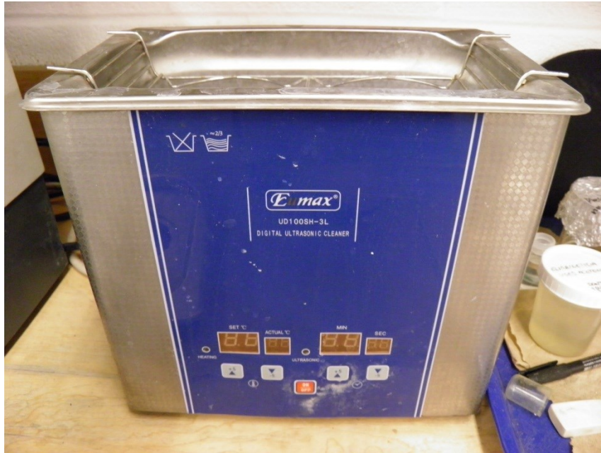
Figure 111: Digital Ultrasonic Bath/Cleaner – Eumax UD100SH-3L
