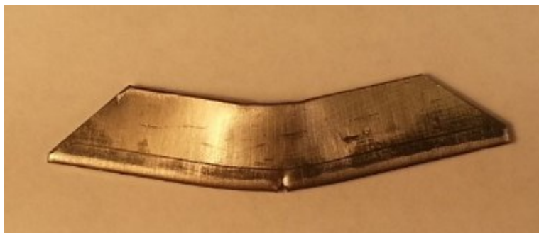
Figure 120: 4-Point Bend Sample (with trimmed edges and crack)
