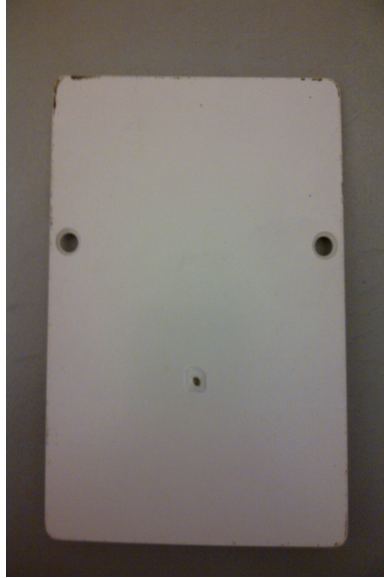
Figure 7.11: Commercially available 915 MHz patch antenna
