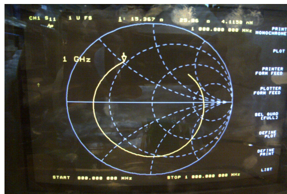
Figure 7.18: Smith chart of network impedance of open platform semi-passive tag
