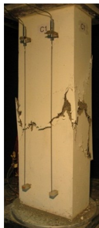
Figure 5.29 Staged Failure Process for Columns with 1%-Fibres
