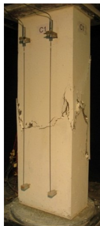
Figure 5.29 Staged Failure Process for Columns with 1%-Fibres
