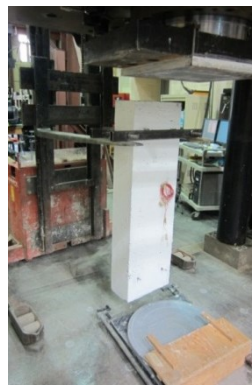
(b) Transferring the column with forklift
