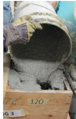
(d) Placing the Concrete into the Formwork
