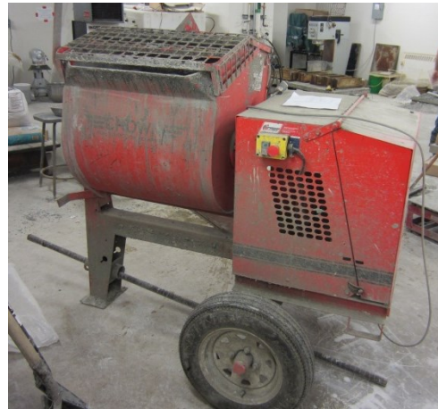
(b) Mortar Mixer Used to Cast UHPFRC
