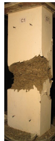
Figure 5.29 Staged Failure Process for Columns with 1%-Fibres
