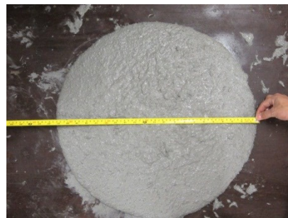
(b) Typical Slump Flow with Fibres (540 mm)
