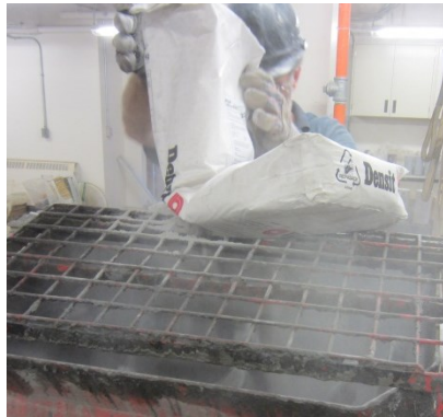
(a) Addition Pre-Packaged CRC and Dry Mixing
