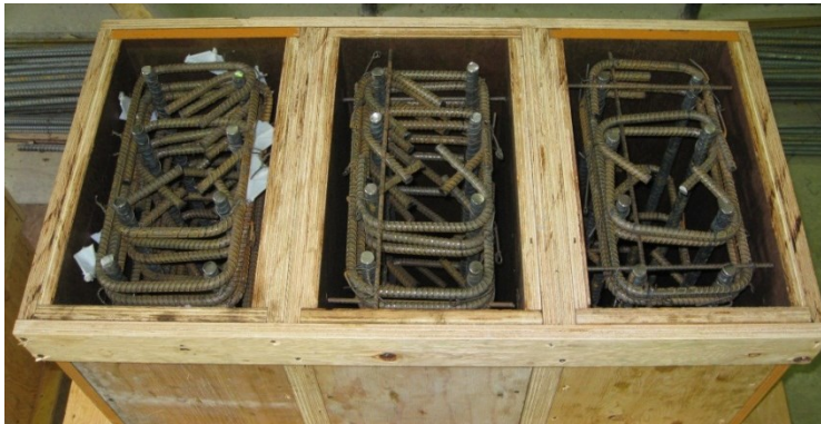
(d)Specimens “With Cover” in Formwork
