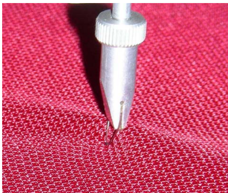
Figure 4.5: Fabric stretching and accumulation and yarn twisting during KES-F roughness measurement
