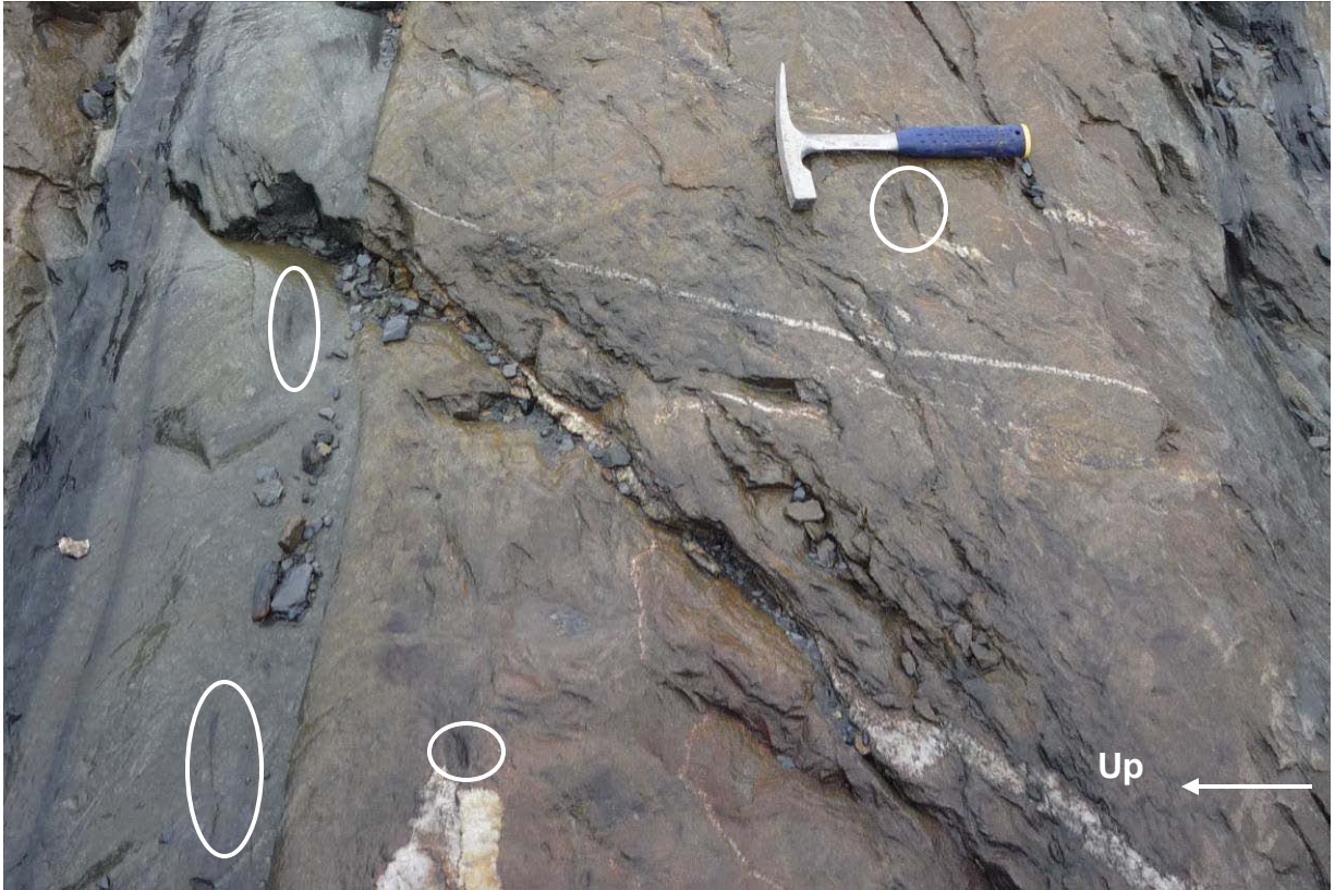
Figure 2.26: Tabular coarse-tail graded structureless sandstone (F3b). Note sharp non-erosive bed bases and isolated tabular mudstone clasts (circled). Note hammer for scale.
