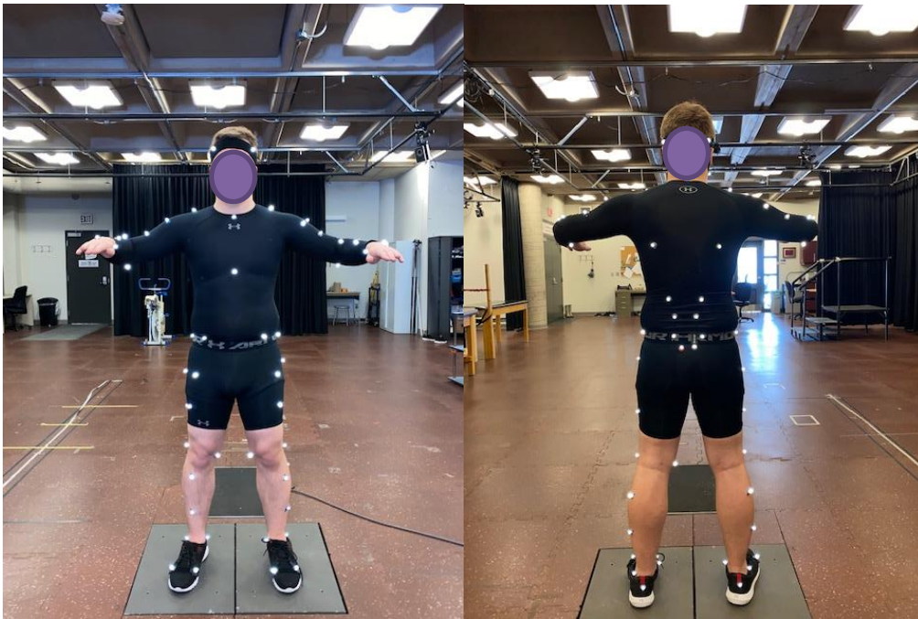
Figure 4-2 Marker configuration and execution of the static pose used in data collections
