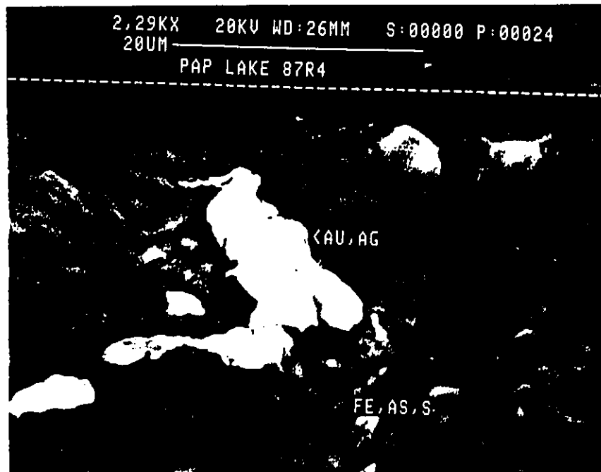
Figure 10. Scanning electron microscope image of primary electron on oxidized arsenopyrite, separated from till overlying the main PAP shear zone.
