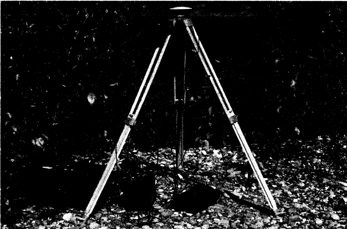
Figure 2-23 RTK-GPS Base; the antenna and Base radio are installed on the top and side of the tripod. The Base receiver is in the black case. A 12V battery provides the power for the system.
