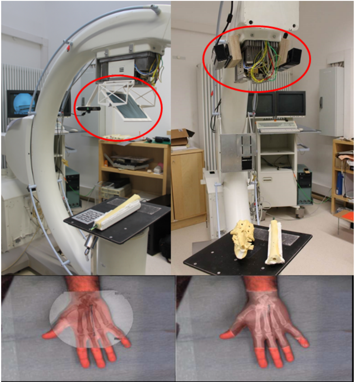
Figure 1.7: Top-left shows a CAM-C system using a video camera, which produces RGB images that can be used for an AR overlay as shown on the bottom. The top-right shows a CAM-C system with depth cameras. Synthetic X-rays can be generated from RGB images taken from video or depth sensors, and from 2-D/3-D point clouds taken from depth sensors [5].
