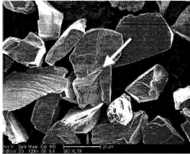
Figure 6.35 Morphology of the SiC particles (the arrow points to a crack in a SiC particle)
