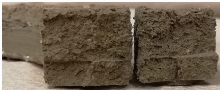
Figure 5.3 Typical shear zone of saturated IHT specimen (IHT3 test, \sigma_n' = 150 kPa)
