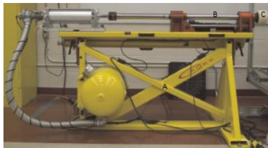
Fig 2. Pneumatic linear impactor frame (A) and impacting arm (B) and striking cap (C).
