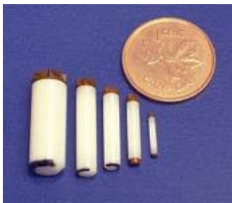
Figure 2.3 Solid NMR rotors. *Most of the samples in this thesis were packed into 7mm (in diameter) rotor.
