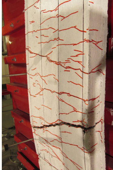
b) CRC-2%A-#3NS-100 Tensile cracking after Blast 4
