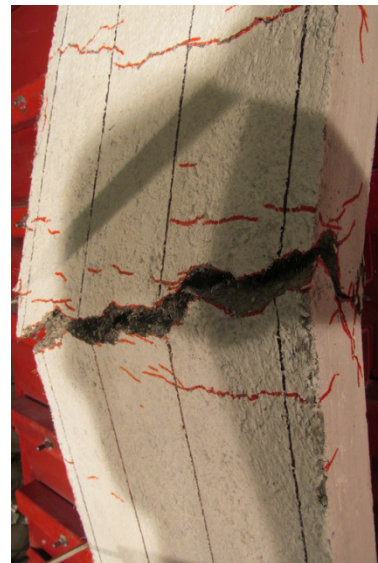
d) CRC-2%B-#3NS-80 Bar rupture at Blast 4
