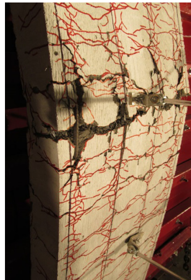
f) SCC-1.2%ZP-#3NS-100 Damage after Blast 5
