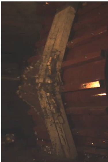
d) SCC-0%-#3HS-100 Excessive fragmentation at Blast 6
