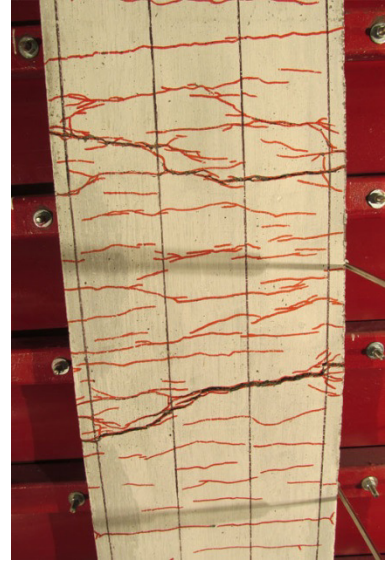
c) CRC-2%B-#3NS-100 Tensile cracking after Blast 4
