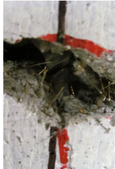
c) CRC-2%A-#3HS-100 Ruptured high strength steel bar
