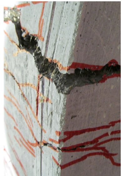
i) Fibres visible at Blast 6
