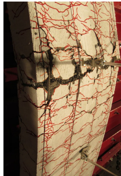
f) SCC-1.2%ZP-#3NS-100 Tensile cracking after Blast 5
