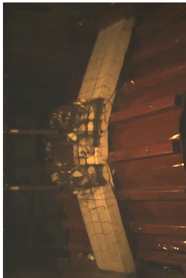
c) SCC-0%-#3NS-100 Excessive fragmentation at Blast 5
