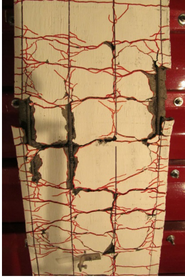
a) SCC-0%-#3NS-100 Damage after Blast 4
