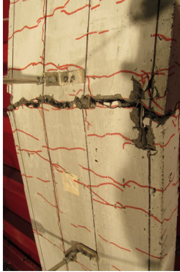
b) SCC-1.2%ZP-6.3NS-80 Damage at Blast 3
