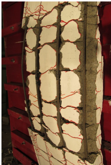
d) SCC-0%-#3NS-100 Excessive fragmentation at Blast 5
