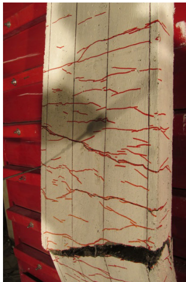
e) CRC-2%A-#3NS-100 Bar rupture failure after Blast 5
