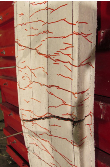
f) Mid-span cracking at Blast 4
