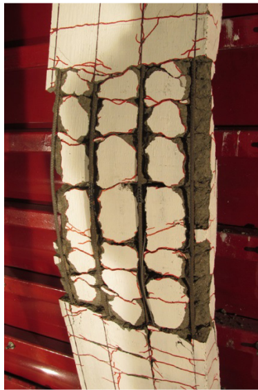
g) Bar slippage and fragmentation at Blast 5
