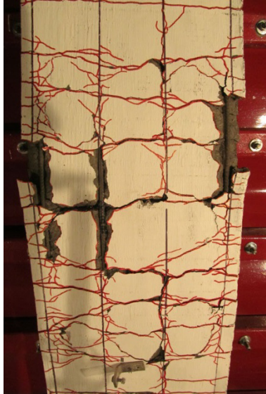
a) SCC-0%-#3NS-100 Damage after Blast 4
