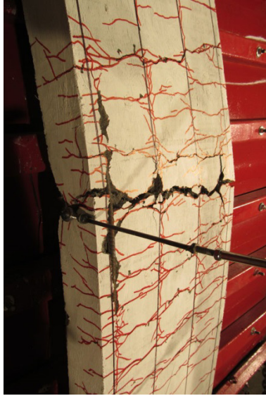
a) SCC-0.6%ZP-#3NS-100 Damage after Blast 4
