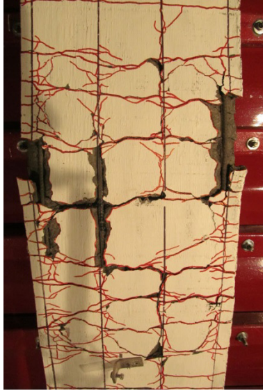
a) SCC-0%-#3NS-100 Damage after Blast 4
