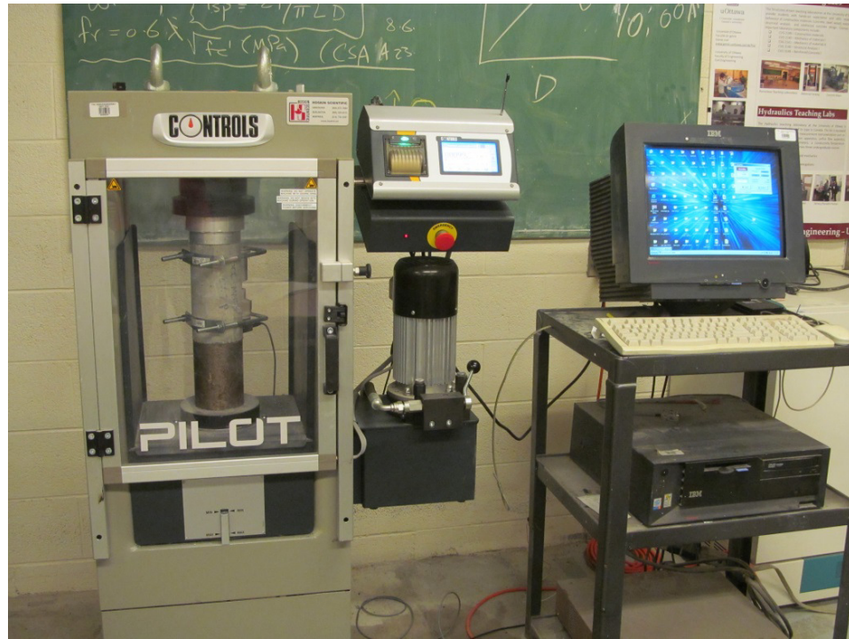
Figure 3-8 Cylinder testing setup
