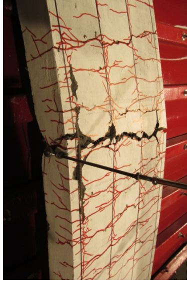
b) SCC-0.6%ZP-#3NS-100 Damage after Blast 4
