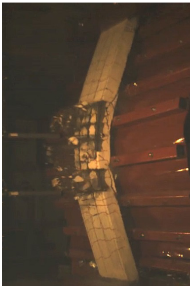
c) SCC-0%-#3NS-100 Excessive fragmentation during Blast 5
