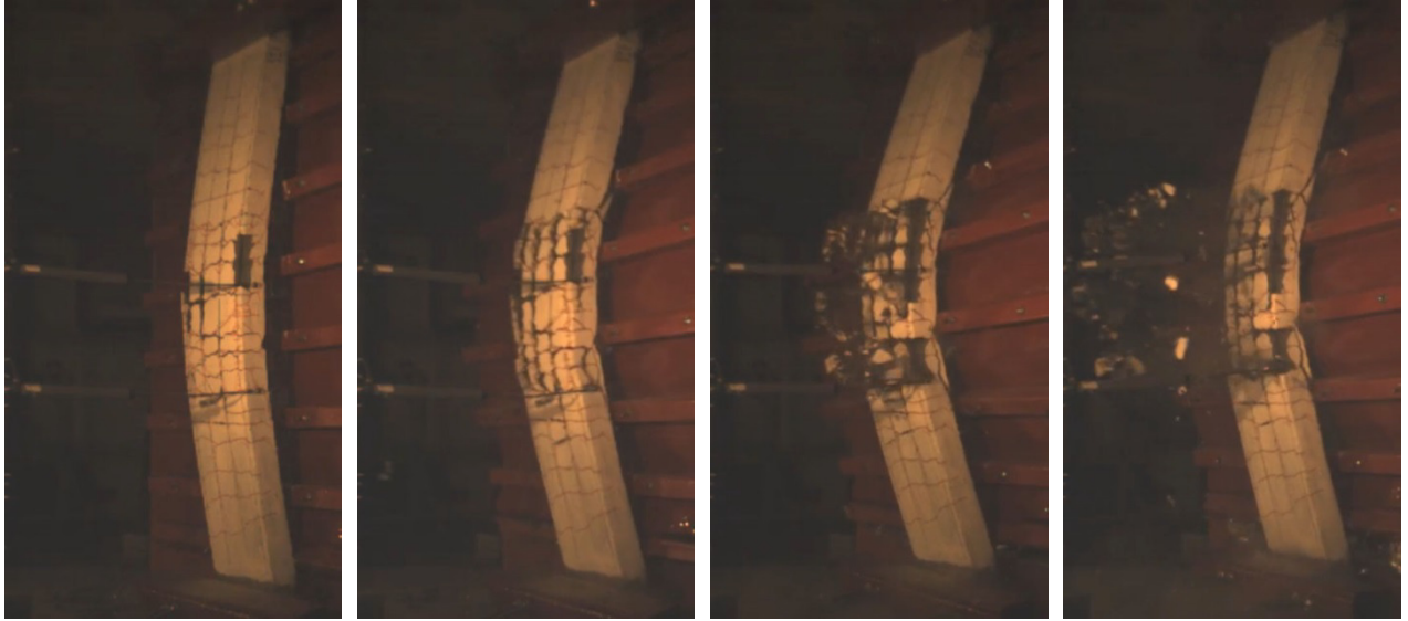
Figure 5-44 SCC-0%-#3NS-100 secondary fragmentation
