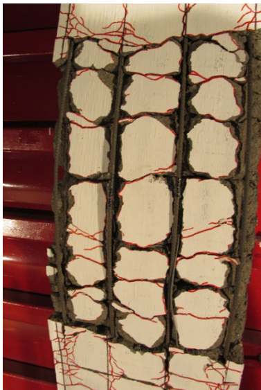
c) SCC-0%-#3NS-100 Bar exposure after Blast 5
