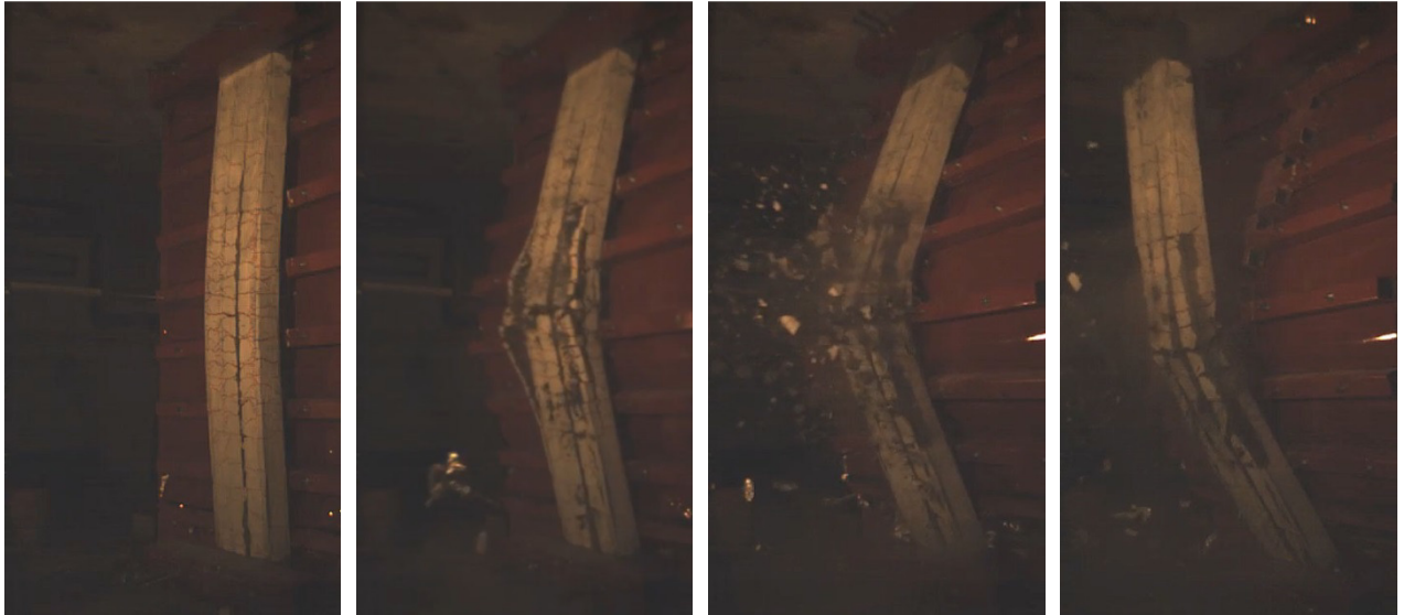
Figure 5-45 SCC-0%-#3HS-100 secondary fragmentation
