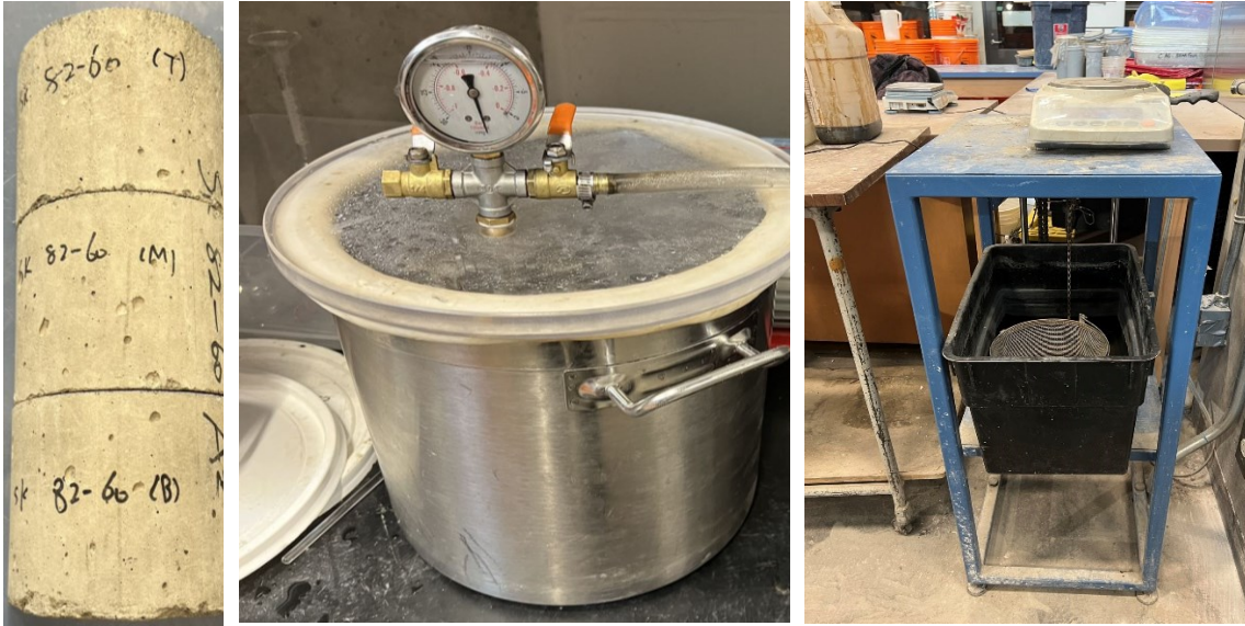
Figure 3.4 Porosity Test: Cutting the Specimen into three parts:(Top, Middle, Bottom), Vacuum Container and Submerged Mass Measurement Table
