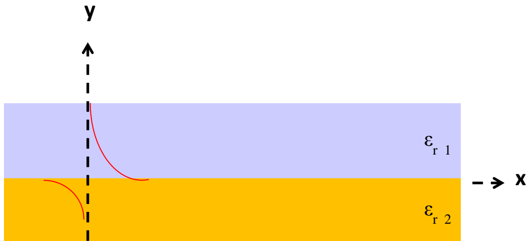
Figure 4: The above figure demonstrates the field strength distribution for a single interface SPP.
