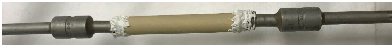
Figure 7.9. Picture showing a membrane attached to the stainless steel tubing of the feed and retentate lines using Torrseal.
