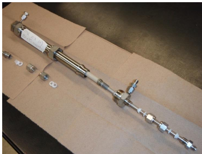
Figure 7.6. Picture showing how the membrane and stainless steel supports assembly is inserted into membrane module 1. Teflon ferrules and Swagelok fittings are used to separate the permeate stream from the feed and retentate streams. The membrane shown in this picture has been attached to the stainless steel tubing of the feed and retentate lines using generic epoxy.
