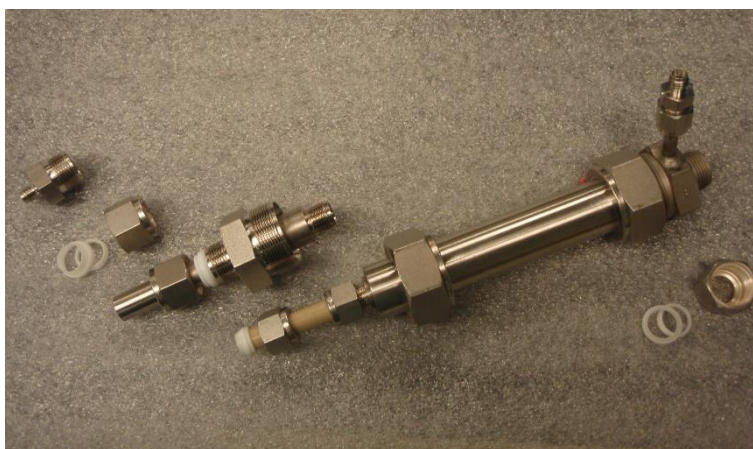
Figure 7.10. Picture showing how the membrane and stainless steel supports assembly is inserted into membrane module 2. Teflon ferrules and Swagelok fittings are used to separate the permeate stream from the feed and retentate streams. The membrane is also been attached to the stainless steel tubing of the feed and retentate lines using Swagelok fittings and Teflon ferrules.
