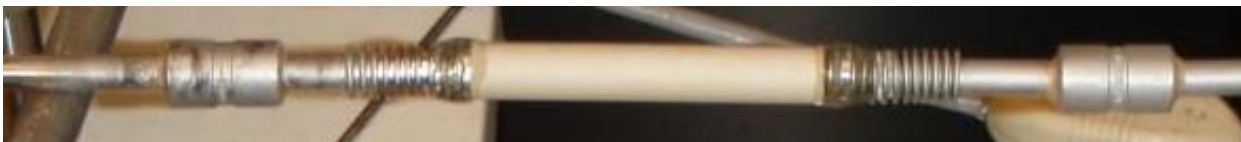
Figure 7.7. Picture showing a membrane attached to the stainless steel tubing of the feed and retentate lines using epoxy.
