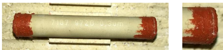
Figure 7.13. Picture showing membrane PP 25 0.3 (1) whose end faces have been coated with silicon rubber on top of Aremco 617. The right hand side picture shows the vertical line where a Teflon ferrule cut at the silicon rubber.
