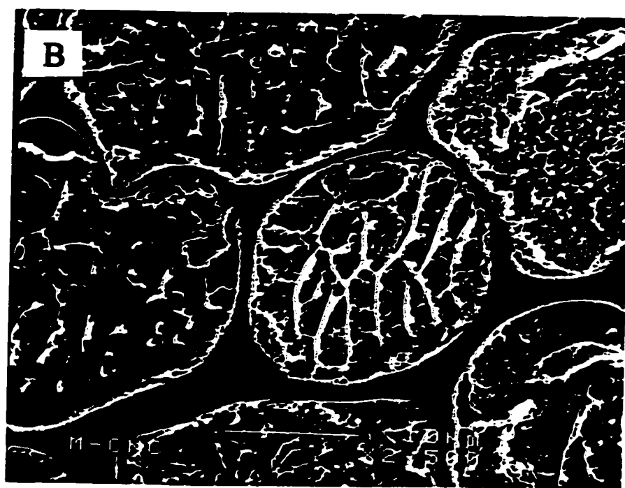
Figure D.2: Scanning electron micrographs (Mag. 2500 ×) of moss cells exposed to (A) \text{Cu}^{2+} - \text{Ni}^{2+} metal system (uptake (mmol/g); \text{Cu}^{2+} : 0.165, \text{Ni}^{2+} : 0.034) and (B) \text{Cu}^{2+} - \text{Ni}^{2+} - \text{Cd}^{2+} metal system (uptake (mmol/g); \text{Cu}^{2+} : 0.150, \text{Ni}^{2+} : 0.025, \text{Cd}^{2+} : 0.041).
