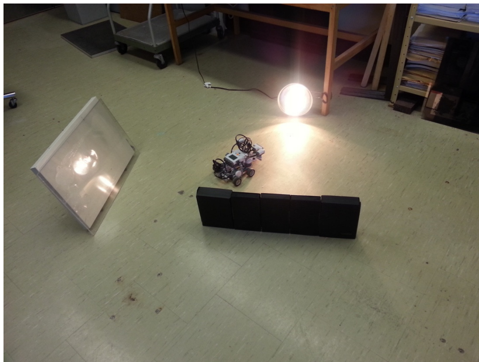
Figure 9. 23 Robot detects higher values of light and temperature as it turns back facing towards a higher value of light
