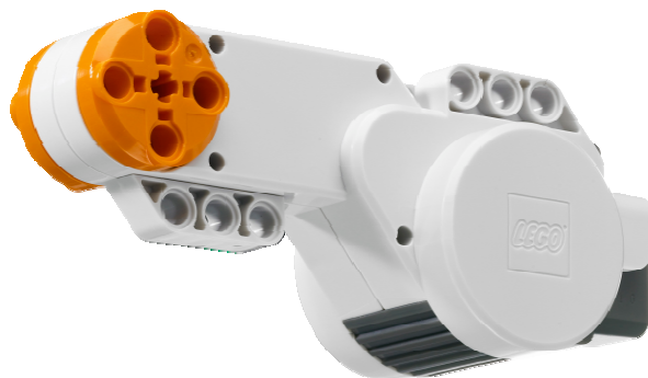
Figure 3.5 Servo Motor with Built-in Rotation Sensor
