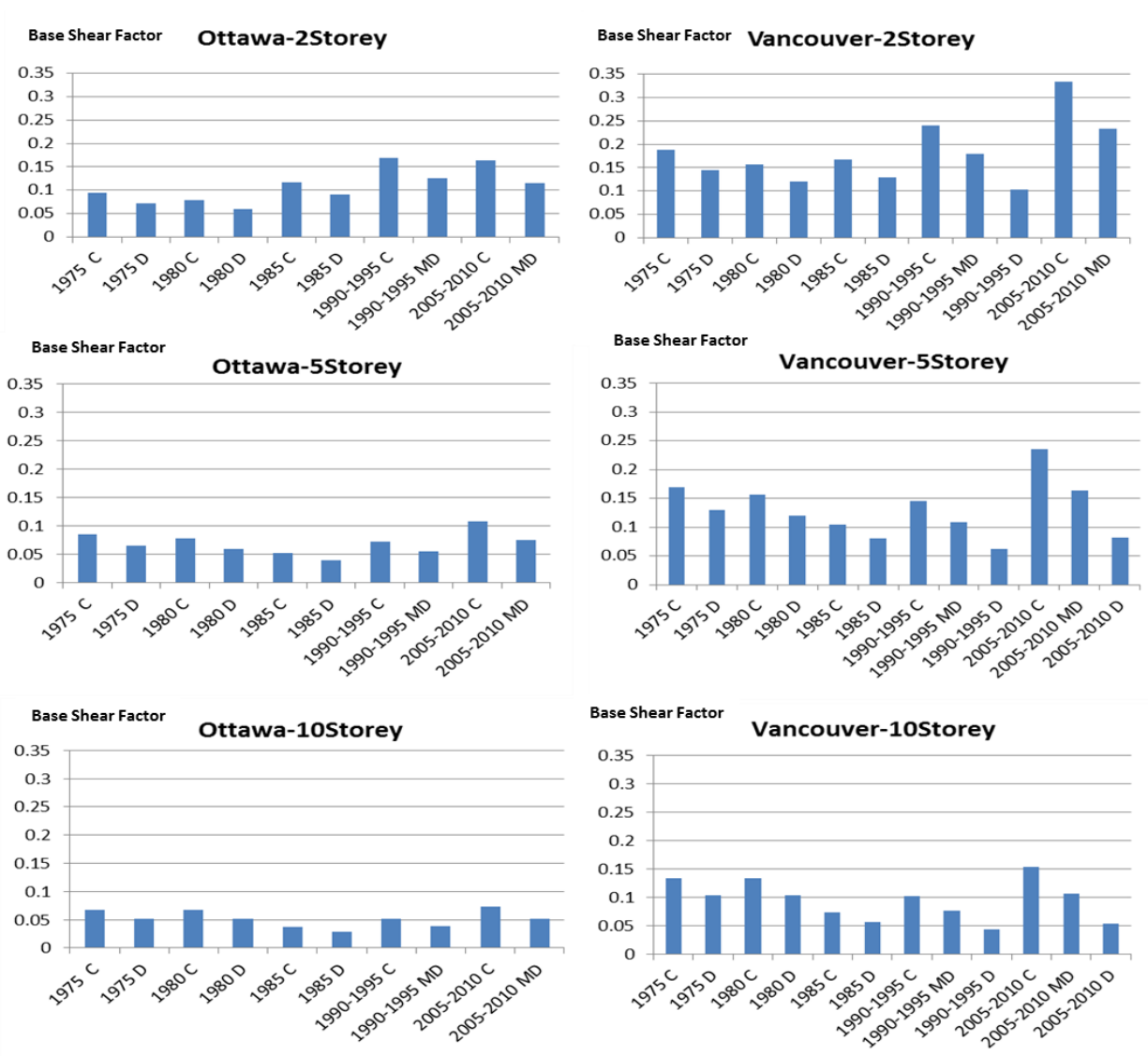
Figure 4-12: Design load level based on different versions of NBCC C: Conventional, MD: Moderate Ductile, D: Ductile
