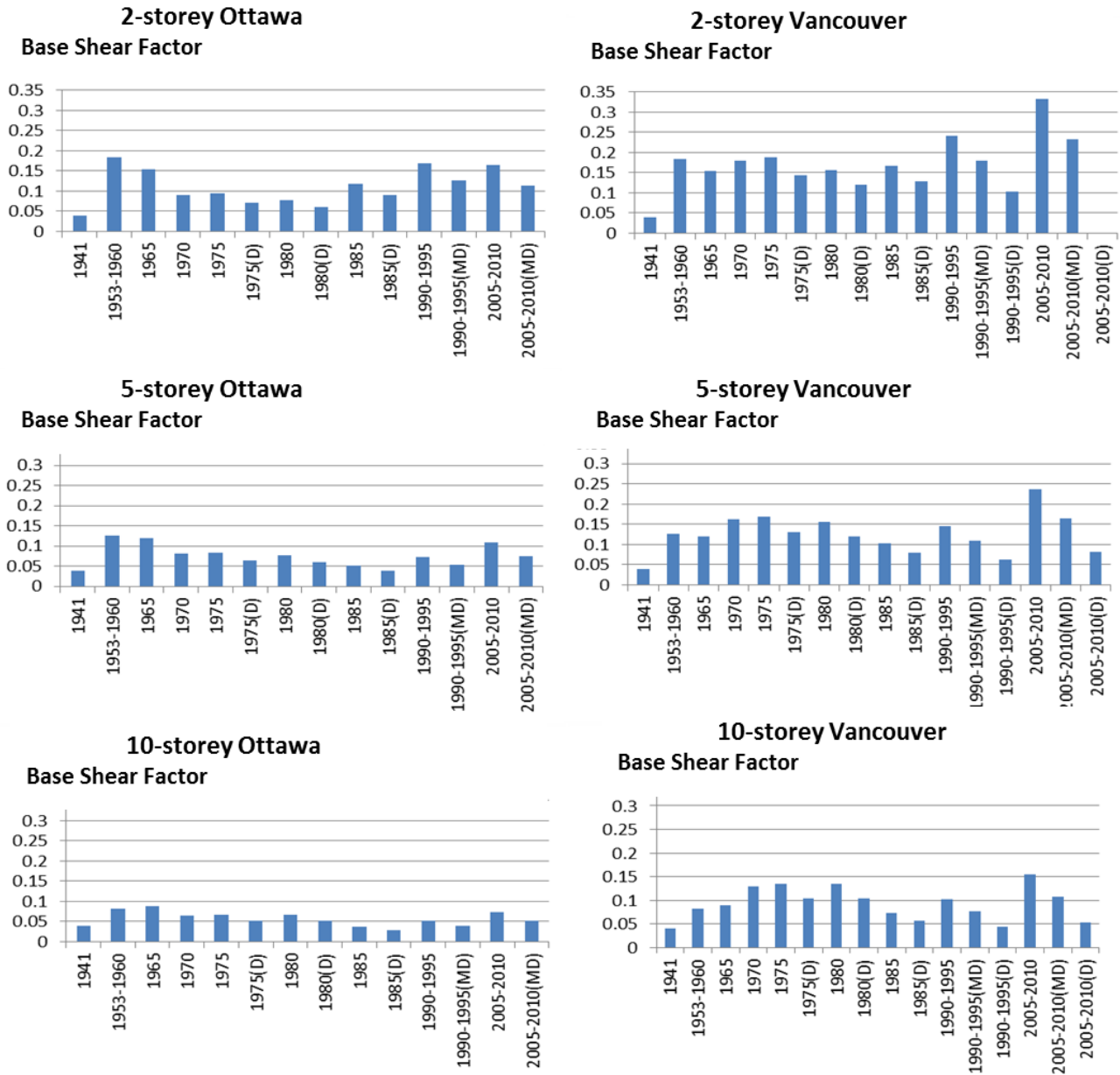
Figure 5-2: Base shear factor of buildings with different height designed based on different codes in Ottawa and Vancouver (MD and D stand for moderately ductile and ductile, respectively)
