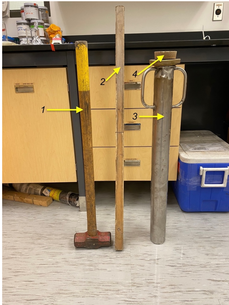
Figure 4. Materials used for soil core collection: 1 sludge hammer, 2 wooden rods, 3 stainless-steel pipes (7.5 cm diameter), 4 wooden disks.
