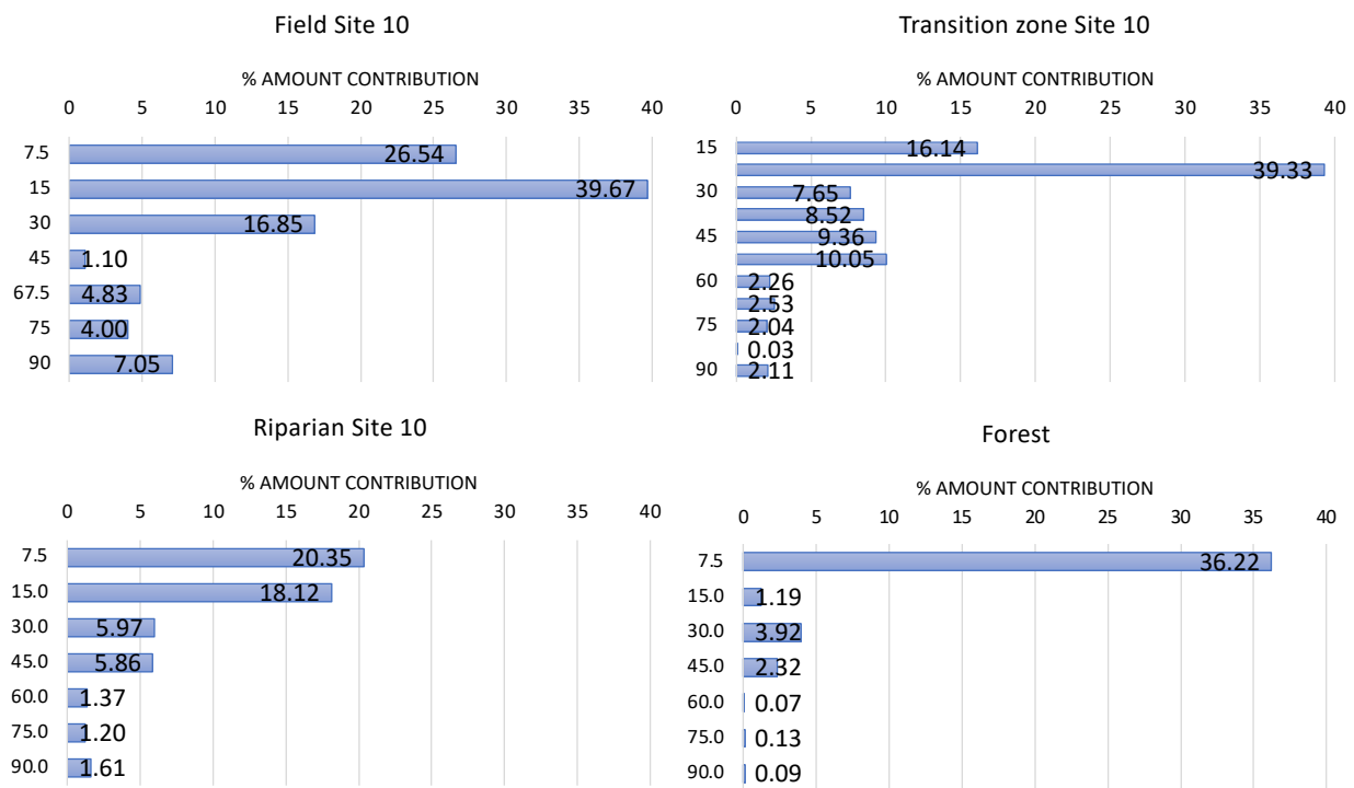
Figure 14. The overall percent contribution of each soil profile depth to the overall percent CO 2 emissions at the surface for study site 10 and the background site. Radiocarbon Fm values were used to calculate the overall percent contribution of each subsequent depth in the soil profile.
