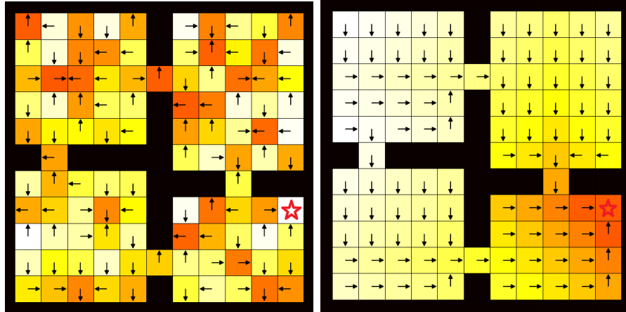
Figure 3.19: Left figure is the arbitrary initialled value function, right figure is converged value function
