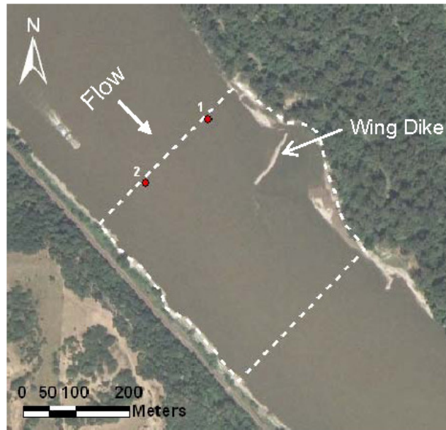
Figure 4.1.1. Aerial photo of the study site in 2005, during low flow conditions. Dashed lines represent the survey extents. Points 1 and 2 indicate locations of stationary measurements.
