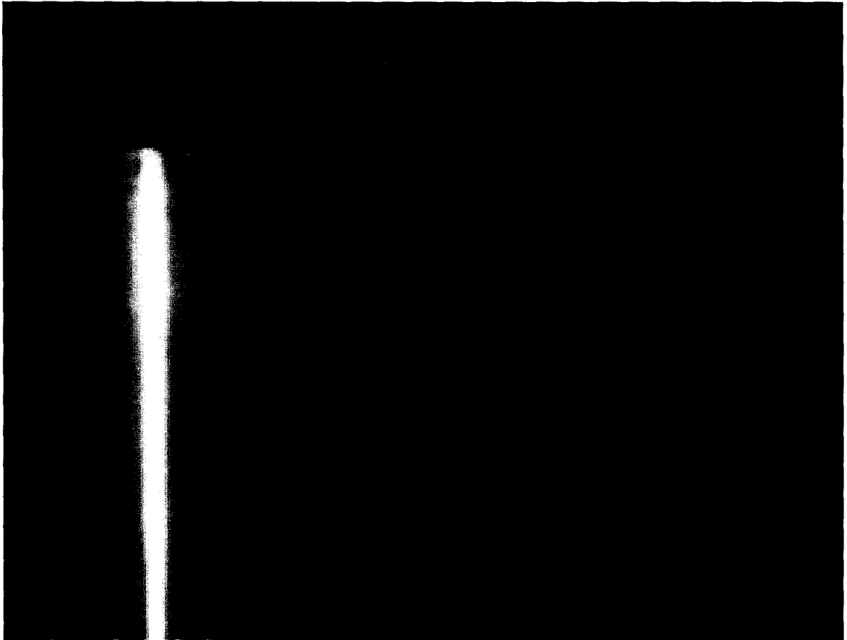
Figure 45 – Image of delayed-regular-mixing-layer-type regime ( d = 22.55 mm, R = 0.050 , Re_j = 469 , Re_\infty = 2349 )
