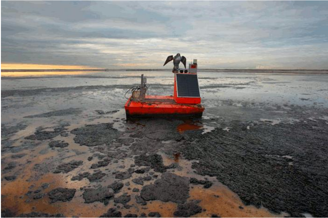
Figure 3: View of a tailing pond in the Athabasca basin. The radar device shown scans for incoming birds and emits a bird of prey call to ward off [source: Peter Essick, National Geographic].
