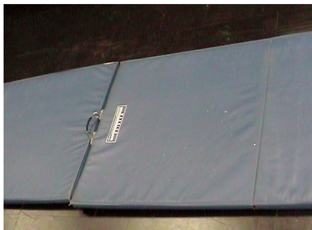
Figure 4: Foam mats used to simulate uneven ground in the thesis.
