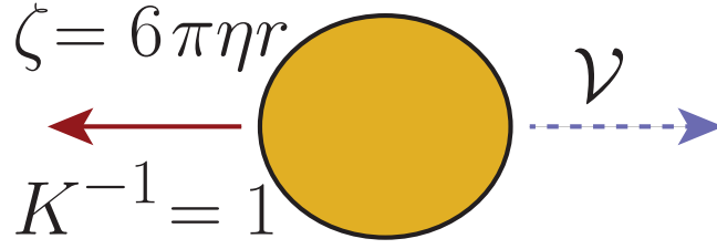
Figure 2.3.5: The drag on a spherical body of radius r moving through a fluid of viscosity \eta at low Reynolds numbers (small speed v ) has a friction coefficient that obeys Stokes' law \zeta = 6\pi\eta r (Equation (2.80)).
