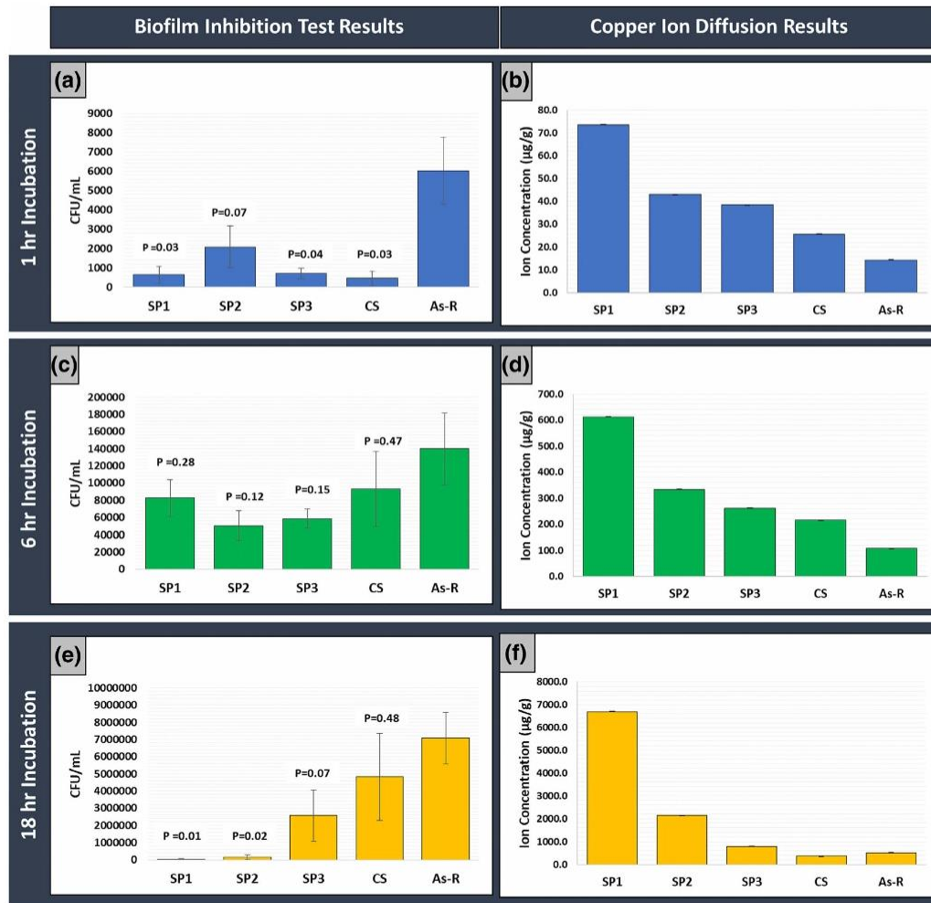
Fig. 6 Pseudomonas aeruginosa bacteria survival in the form of microcolonies and biofilm reported in “CFU/mL” at (a) 1 hr, (c) 6 hr, and (e) 18 hr incubation time. The copper ion released from the samples reported in “µg/g” is shown at (b) 1 hr, (d) 6 hr, and (f) 18 hr
