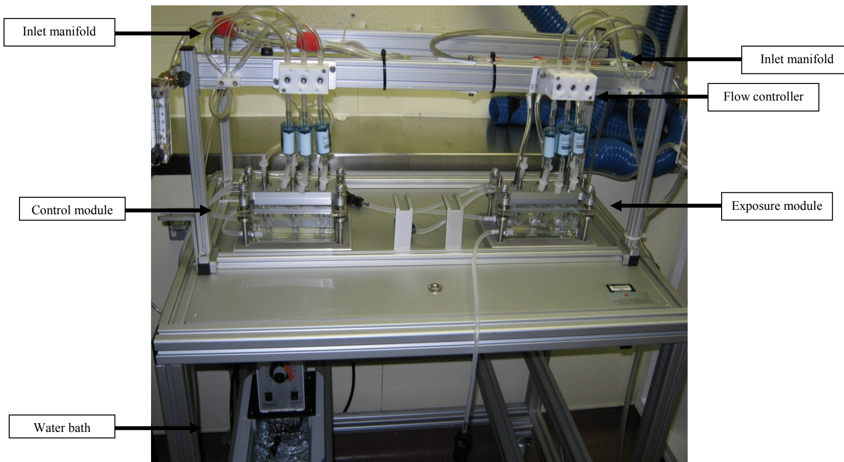
Figure 2.1: Front view of the cart-mounted VITROCELL® system. The aerosol exposure module with above inlet manifold is shown at the right. The matching control (i.e., clean air) module is shown at the left. The water bath for temperature control is below. The vacuum pump is not shown.
