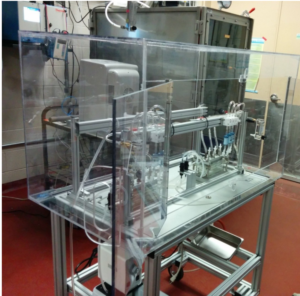
Figure 2.7: Plexiglas box built to maintain temperature.
