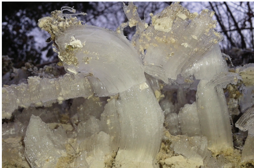
Figure 7. Needle ice formed in fine-grained soil in Chiltern Hills, UK during two nights of frost (Gibbs, 2014)
