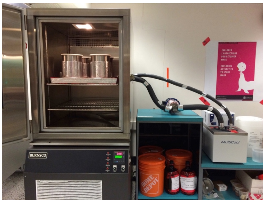
Figure 15. Assembled setup: Environmental chamber with the four cooling plates connected to the pump and the cold bath located in the Cryolab for Arctic, Antarctic and Planetary Studies.
