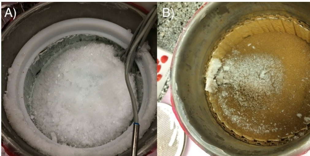
Figure 30. Picture of vapour deposited hoar frost on top of the glass beads (A) and the JSC Mars-1 experimental soil (B)
