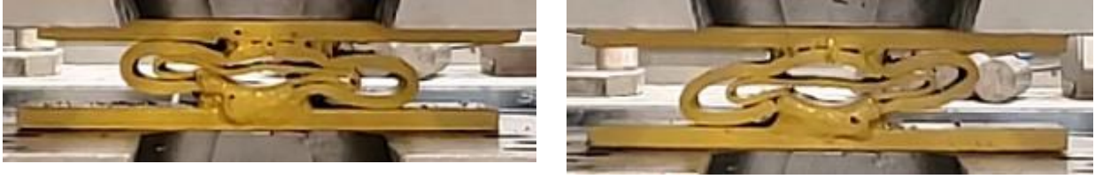
(ii) Deformed Shape
