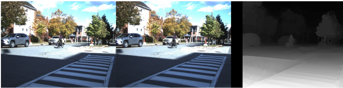
FIGURE 2.7: A sample of generated disparity maps. Left: images taken from both stereo cameras. Right: disparity map. Darker the color, further the object.
