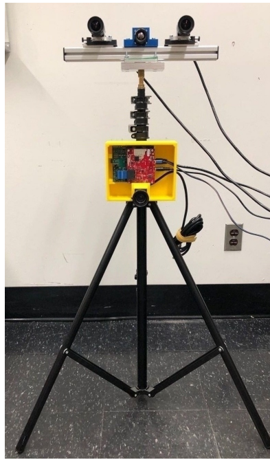
FIGURE 4.1: Sensors setup: Stereo camera DFK 33UX273 is fixed at the top of the tripod; AWR1843Boost radar is installed in a yellow box which is attached to the middle of the tripod.
