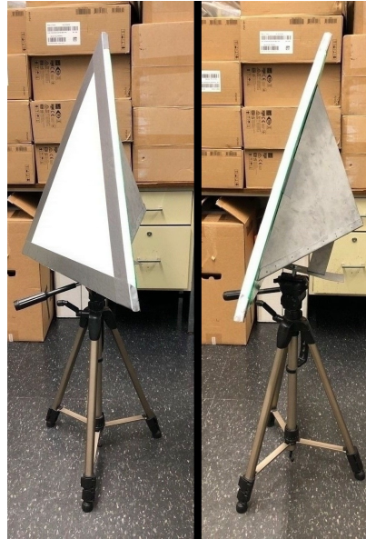
FIGURE 4.2: Calibration target: a triangle shape styrofoam attached to a trihedral corner reflector.
