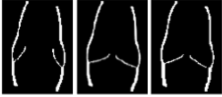
Figure 30: Image warping from time step 7 to time step 1 using demons method with the built in pyramid scheme: time step 1 (left), warped image 7 to 1 (middle), time step 7 (right)
