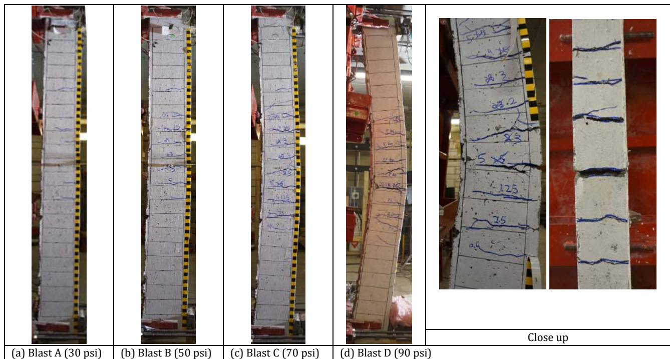
Figure 5-10 – HSC-F0.75-15M-10M-d/2 - Photographs at the end of Blasts A, B, C and D
