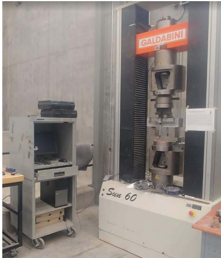
Figure 3-12- GALDABINI SUN 60 Universal Floor Standing Testing Machine
