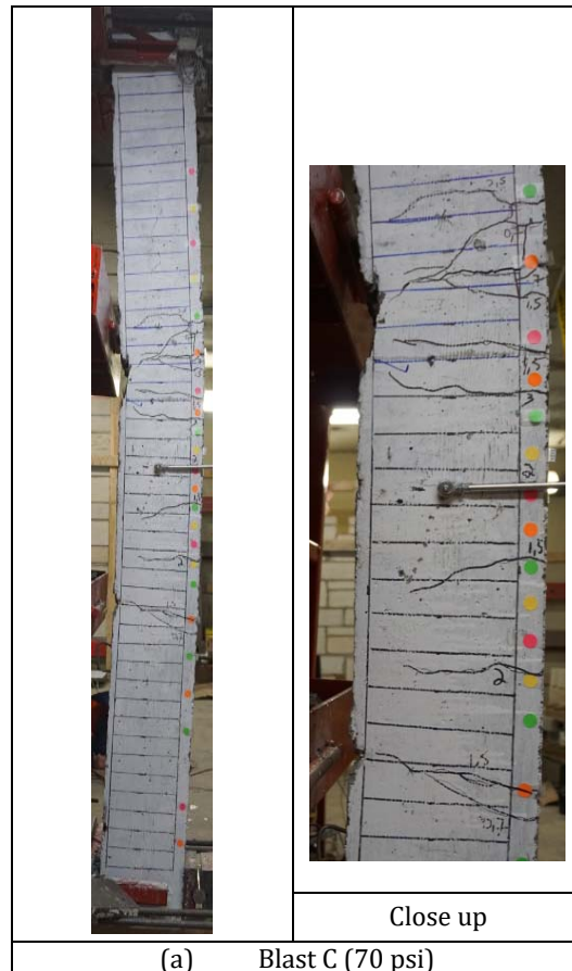
Figure 5-6 - HSC-F0-15M-10M-d/4[x1] - Photographs at the end of Blast C
