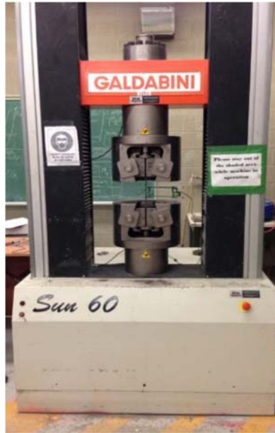
Figure 3-3 - Galdabini Steel Coupon Testing Setup
