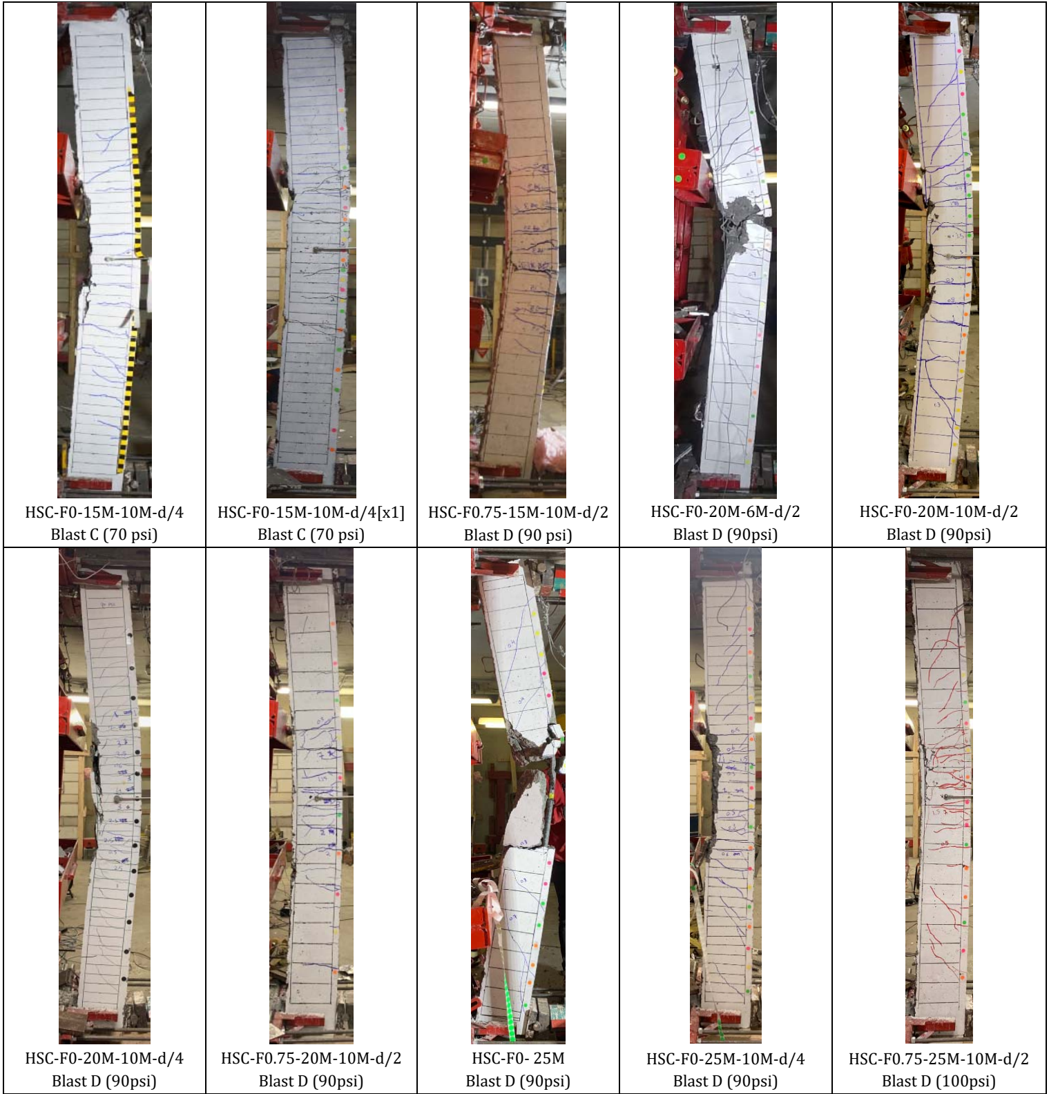
Figure 6-4 –Photos of all beams indicating Final Blasts
