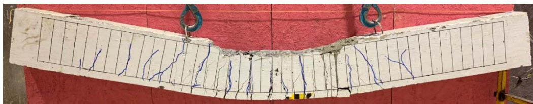
Figure 6-25 – Residual test results for beams tested under single and repeated blasts
