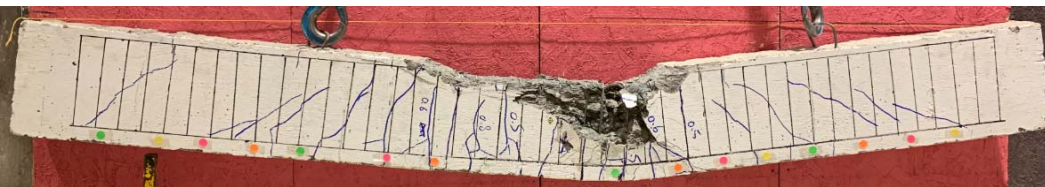
Figure 6-34 – Residual test results for beams tested Effect of reinforcement ratio (HSC beams)
