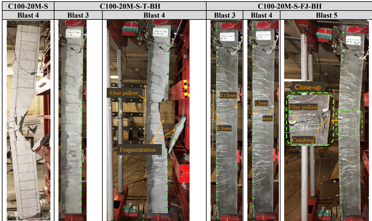
Figure 6 - 11 Damage profiles of specimens with 20M and stirrups
