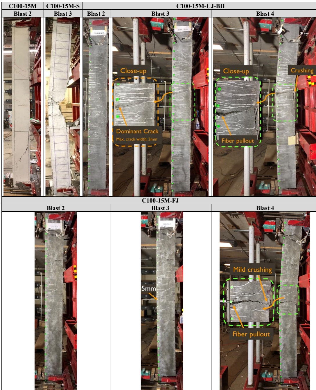
Figure 6 - 7 Damage profiles of specimens with 15M
