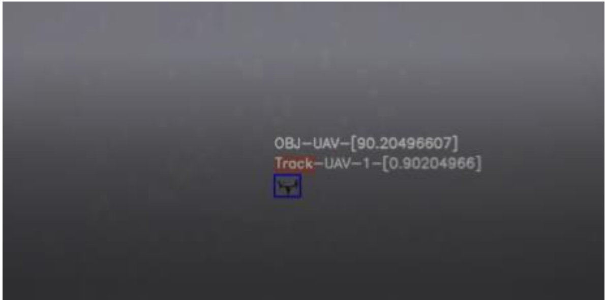
Fig 5- 16. YOLOv3 tracker made the detection with 90% confidence.
