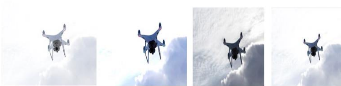
Fig 4- 15. The original image was subjected to different transformations, with a brightening level of 100, a contrast level of 56, a darkening level of 199, and a deepening level of 100.
