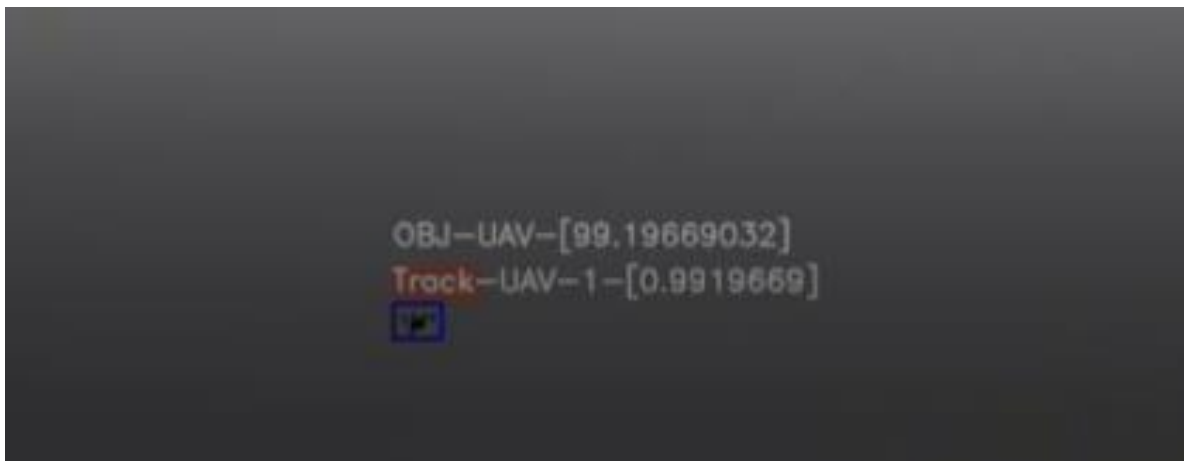
Fig 5- 17. YOLOv3 tracker made the detection with 99% confidence of a tiny drone.
