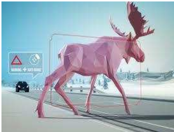
Figure 2.6: On-vehicle animal detection system. Camera captures the dangerous animals which are crossing the road, and the system recognizes the target and warns drivers about the imminent danger.
