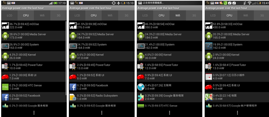
Figure 7.7: Average Power consumption over 60 minutes ( mW ): from left to right are shown HOG+AdaBoost, LBP+AdaBoost, Haar+AdaBoost and HOG+SVM. We can see that other system applications such as “Media Server”, “System”, “Kernel”, and “Power Tutor”, consume quite limited and similar power usage over the last 60 minutes.
