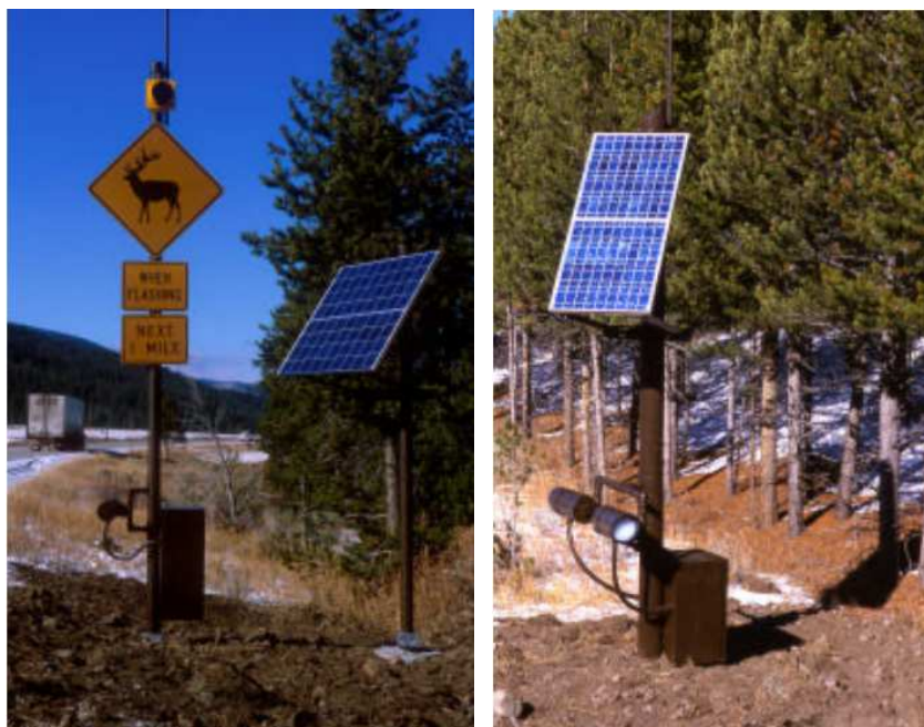
Figure 2.4: Roadside dynamic animal sensor system example (Photo courtesy of the Western Transportation Institute) [22]
