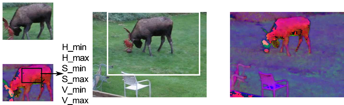
Figure 6.18: RGB image & HSV image. Only the body part (black rectangle in the left-bottom image) was selected to calculate the HSV filter values. The white rectangle in the middle image is the ROI determined by the last frame detection result.
