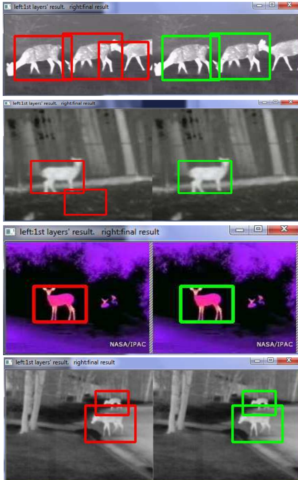
Figure 6.23: Nighttime experimental results performed on still images. Left window: the output of the first classifier; Right window: the detection result of the overall classifier.
