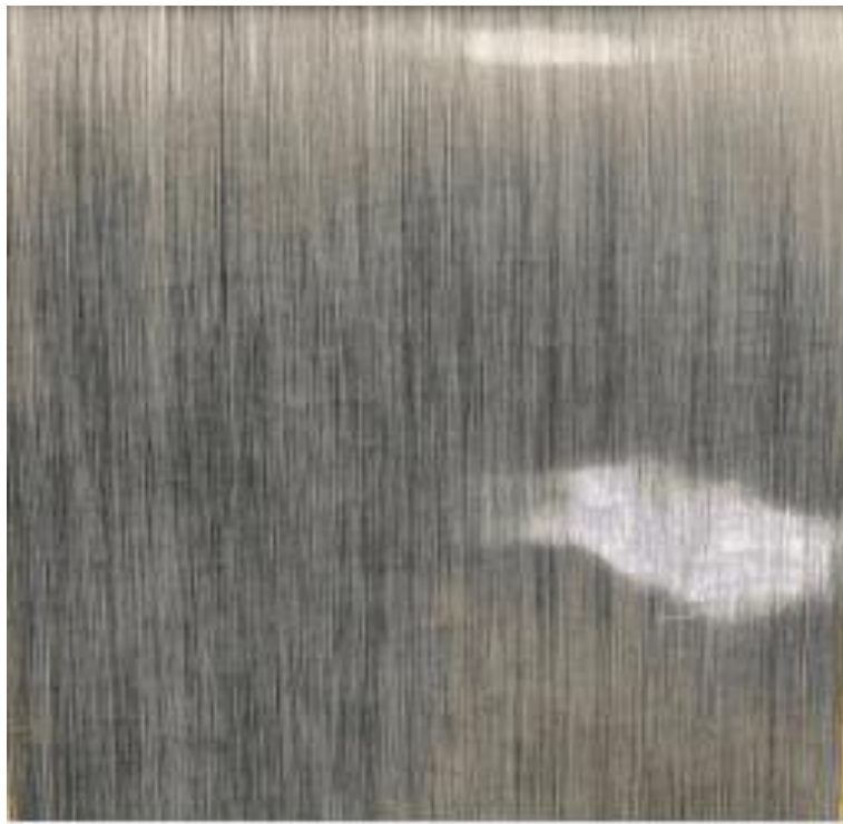
Figure 5.2 Unidirectional prepreg with no visual defects
