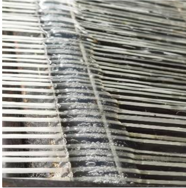
Figure 4.6 Photograph of glass fibres impregnated by PP polymer inside the impregnation mould
