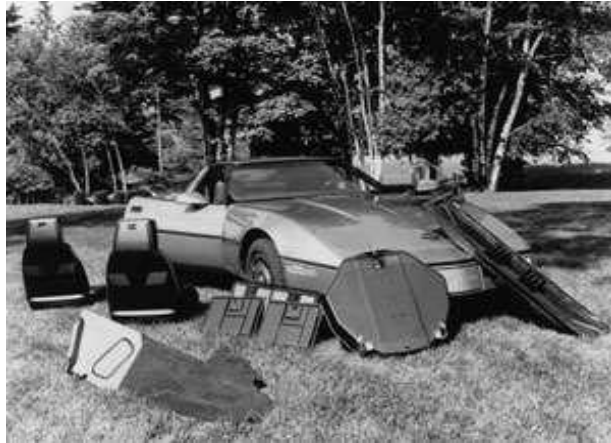
Figure 2.6 GMT parts used in C4 Chevrolet Corvette produced from 1983 to 1996 [34]
