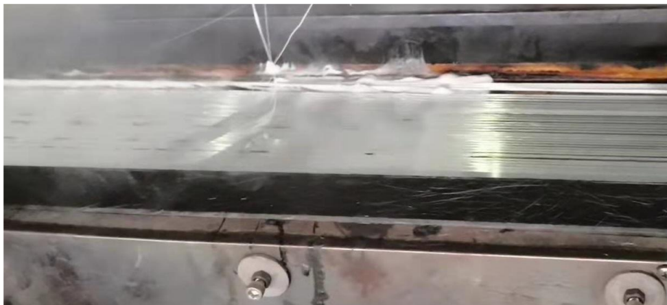
Figure 4.7 Photograph of tests of the impregnation mould and process
