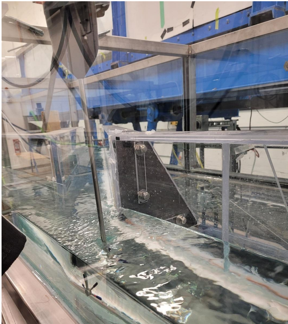
Figure 64. Acoustic Doppler Velocimetry (ADV) to verify flow conditions
