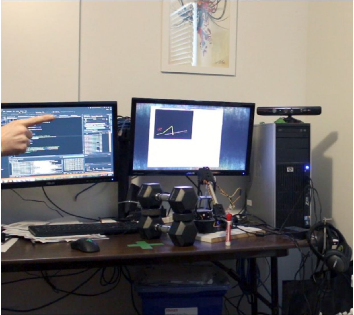
Figure 50 After going back on the other side of the obstacle through the opening with the marker inside the gripper's jaws, the user adjusts the posture of the robotic using the attraction point method arm to place the marker vertically on the table.
