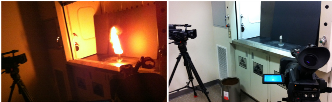
Figure 15: The setup for capturing small-scale flames in a fume hood cabinet
