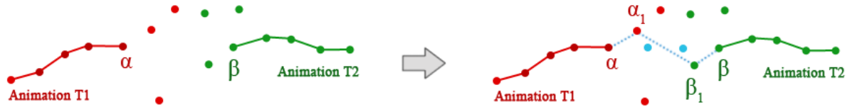
Figure 36: The concept of Direct Bridging method, visualized in 2D. The image on the right shows connection of \alpha to \beta using this method for N=2 steps. Two temporary data points (in blue) are first inserted between \alpha and \beta to build a bridge, and then we look for the nearest points to each of them that form a path illustrated with blue dotted line
