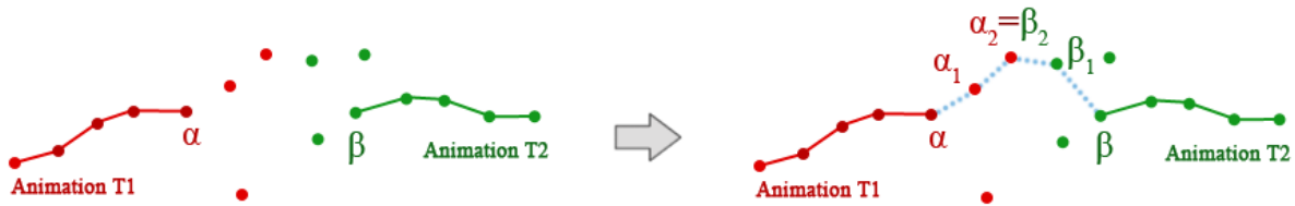
Figure 38: The concept of End Growing Connection method, visualized in 2D. The blue dotted line is our optimized path using algorithm 1, and although a maximum N=20 steps is chosen the algorithm stops in three steps by finding a shared image ( \alpha_2 = \beta_2 )
