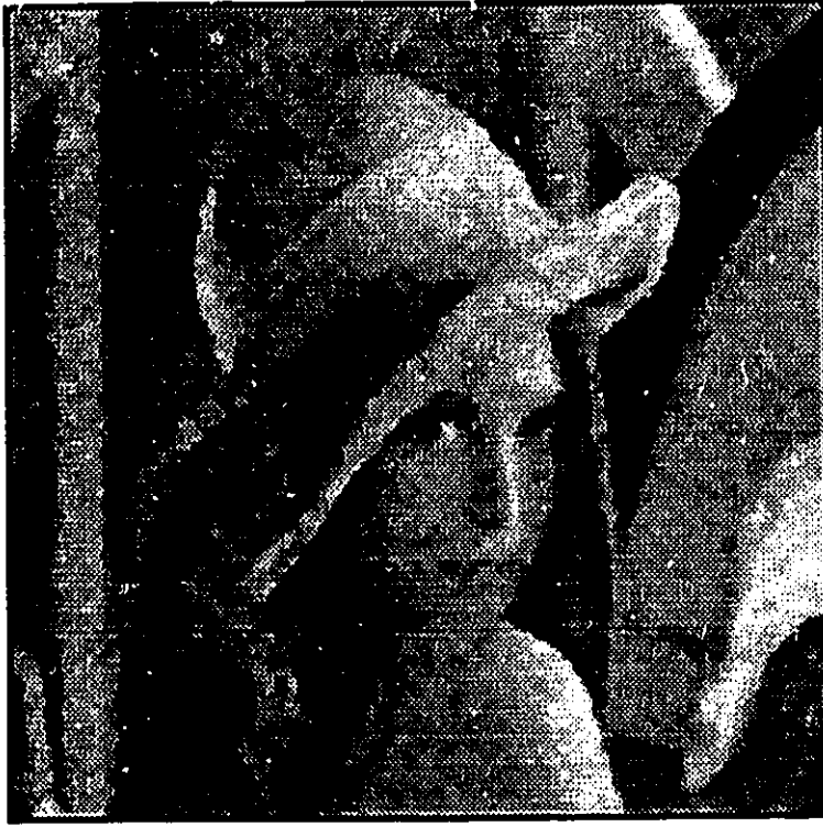
Figure 5.12: CST encoded Lenna image reconstructed at 0.078 bits per pixel
