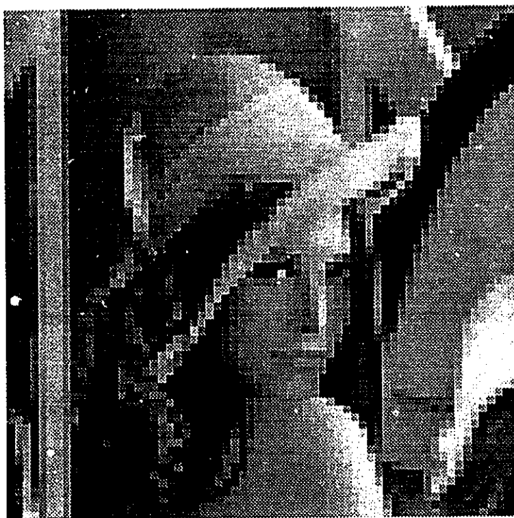
Figure 5.10: JPEG-DCT encoded Lenna image reconstructed at 0.08 bits per pixel
