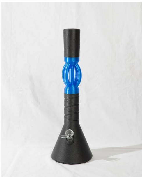
Figure 3.4 3D printed part which could be tested in parallel or in perpendicular to the printing axis [79].
