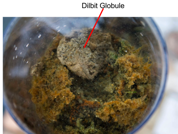
Figure S4. Example of a tarball sitting on top of the sediment in a coring tube. The tarball was removed and then the top 1cm of the core was processed for PAC analysis.
