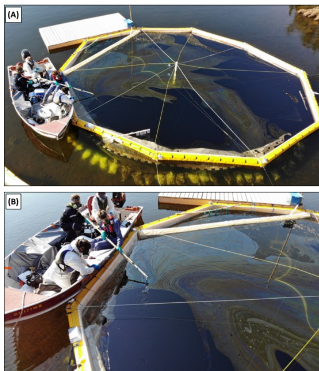
Figure S2. The addition of 180 L of CLWB (1:500 oil:water, v/v) onto the water surface of the limnocorral. (A) Overview of addition method and visible sandbags used to seal the membrane to the sediments, (B) View of telescopic arm and pumping system being held at approximately 5–10 cm from the water's surface. The oil exited the hose parallel to the water's surface to avoid forcing oil below the water surface and allowing it to spread out during the addition.
