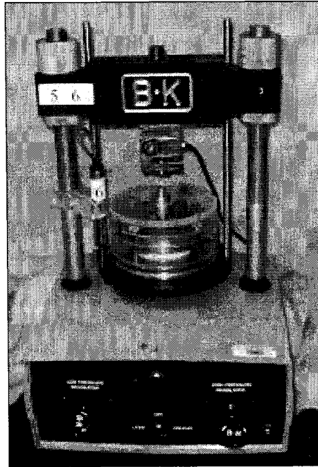
Figure 3.10: Brainard and Kilman oedometer machine.
