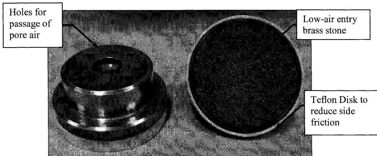
Figure 3.7: Loading cap for oedometer including low-air entry brass stone and Teflon ring.
