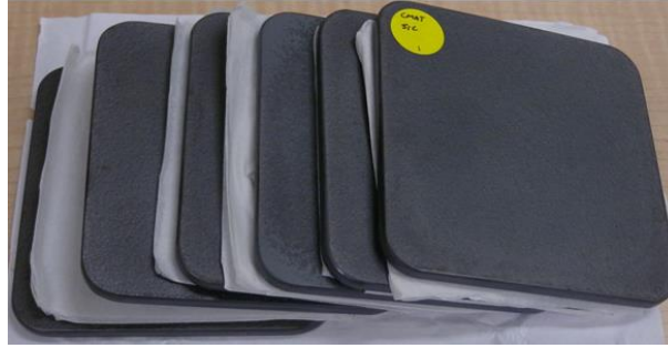
Figure 3.3: Picture of a set of the ceramic tiles showing chamfer edges.
